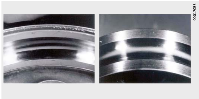
Figure 3 Marks on raceways
