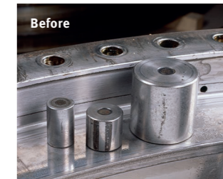
Rollers and raceway with corrosion marks and foreign body indentations
