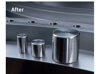
Reground raceway, new rollers with adjusted oversize
