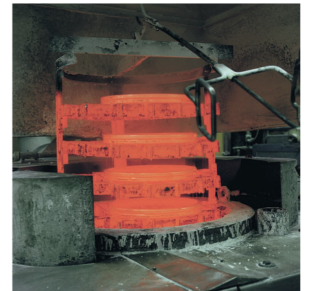
Case hardening ensures increased wear resistance and fatigue strength
